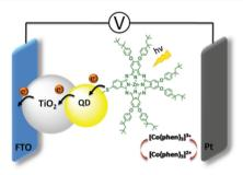
The cascade co-sensitization concept is demonstrated by the sensitization of TiO<sub>2</sub> electrodes with CdS quantum dots (QDs) covalently linked to zinc phthalocyanines (ZnPcs) via a sulfur atom. The efficiency of co-sensitized CdS QD-SZnPc cells, using Co(phen)<sub>3</sub>]<sup>3+</sup>/[Co(phen)<sub>3</sub>]<sup>2+</sup> as electrolyte, is 212% higher than that of a solar cell sensitized just with CdS QD.
