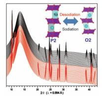
The phase transition of a sodium layered material with P2 stacking during electrochemical desodiation/sodiation studied by in situ synchrotron X-ray diffraction using a capillary-based microcell.  $P2-Na_{0.7}Fe_{0.4}Mn_{0.4}Co_{0.2}O_2$  is transformed to an O2 structure in the voltage plateau at 4.1 V, and the O2 phase shows a rapid change in the c lattice until a fully charged state.
