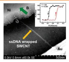
Spin filtering through single-wall carbon nanotubes (SWCNTs) wrapped with single-stranded DNA is demonstrated. Significant spin polarization, larger than typical transition metal ferromagnets, is observed at low temperatures. The helical wrapping of the ssDNA induces an inversion asymmetric electric field in the SWCNT channel, which results in a Rashba-type spin-orbit interaction and polarizes carrier spins.
