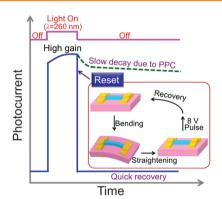
A single SnO<sub>2</sub> microrod photoconductor is demonstrated on a flexible substrate with the photoconductive gain as high as  $\approx 1.5 \times 10^9$ . More interestingly, the recovery time can be reduced from more than 1 d to less than 1 s by a novel "reset" process: bending and straightening the microrod and subsequently applying a voltage pulse.
