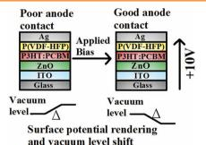
Poly(vinylidenefluoride-hexafluoropropylene) (P(VDF-HFP)) is demonstrated as an efficient buffer layer in cathode/ anode interface of conventional/inverted solar cells, with tunable dipole rendering surface potential of active layers. Integer charge transfer (ICT) model is employed to unveil the effect of surface potential on electrode contact and device performance. Understanding the function of dipole makes P(VDF-HFP) a versatile buffer layer for PSCs.
